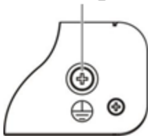
Figure 2-1 Grounding of the RG-NBS3100
